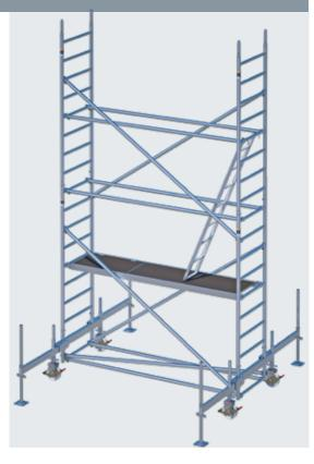
• Fit 2 aluminium guardrails 2600 3.00 m (12 rungs) above the decked surface (The operative has to ascend in such a way that she/he is always secured by the guardrail pair already mounted at a height of at least 1.00 m above her/ his standing height)
