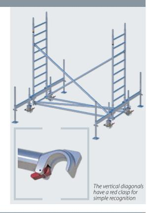
• Fit 2 aluminium guardrails 2600 to the uppermost ladder rung
